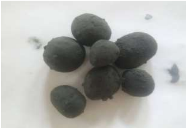
Fig 1. ALWA produced using both POFA and FA after 28 days of curing
